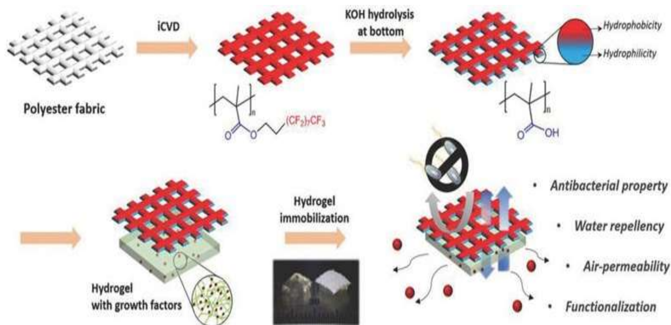
Figure 4: A schematic illustration that shows the fabrication steps of gelatin methacrylate (GelMA) hydrogel-immobilized Janus membrane and in-vivo skin regeneration [Source: Adv. Healthcare Mater (2017)].
